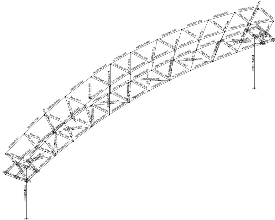
Figure 2: Bridge Sizes Isometric
